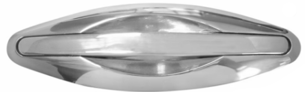
#93.104 Pop up Cleat; Foot print: 10 inch x 2.38 inch. (Slim line 304). Spring Loaded. Pops up by pushing button. Finish: Polished Stainless Steel.
