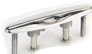
#93.104 Pop up Cleat; Foot print: 10 inch x 2.38 inch. (Slim line 304). Spring Loaded. Pops up by pushing button. Finish: Polished Stainless Steel.
