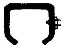
Connecting bracket #54.234 for rail #7 With set screws
