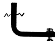
#54.821 No. 8 rail to wall bracket
