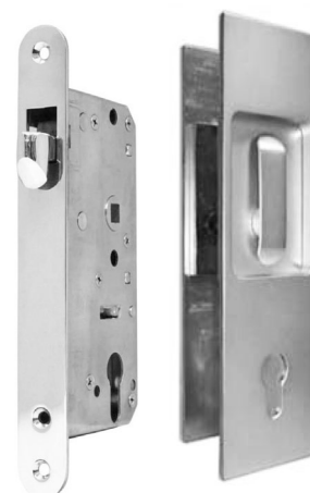
Entry Lock Set#13.81Z6; 55 mm backset; Flush lever set: #13.610Z Minimum door thickness this set up: 42 mm or 1 3/4 inch
