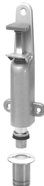
#32.1038.508 Door holder, Push type Throw: 30 mm #32.1038.308 Polished Stainless steel use with in Floor Receiver #32.K42 STAINLESS STEEL
