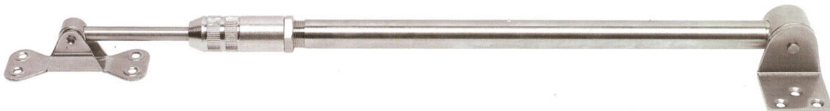
#32.500.508 telescopic stay; stroke: 225 mm. Stainless steel. For medium heavy doors up to 80 lbs.
