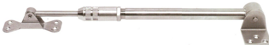
#32.500.508 telescopic stay; stroke: 125 mm. Stainless steel. For medium heavy doors up to 80 lbs.
