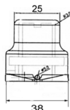
#24.5305 I backset 235 mm. Cut to custom size. (dimensions in mm)
