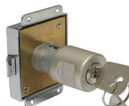
latch #21.711Z; 30 mm backset, brass chrome plated
