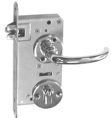
#10.9345Z.308 Set: Entry lock 55 mm backset, with lever #18.956, roses #14.304.
