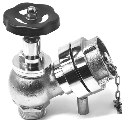
#91.777 Valve 1 1/4" showing with Storz coupling and dust cap N=52 Steel powder coated turning wheel Thread: 1 1/4" BSP. Valve chrome plated brass
